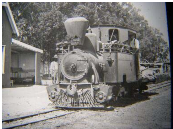
The Orenstein & Koppel 150HP Wood Burner 0-8-0 of 1907 South Western Railway Co Knysna 2 ft Forest Railway – www.herman.rula.co.za (photo Hannes Paling)
