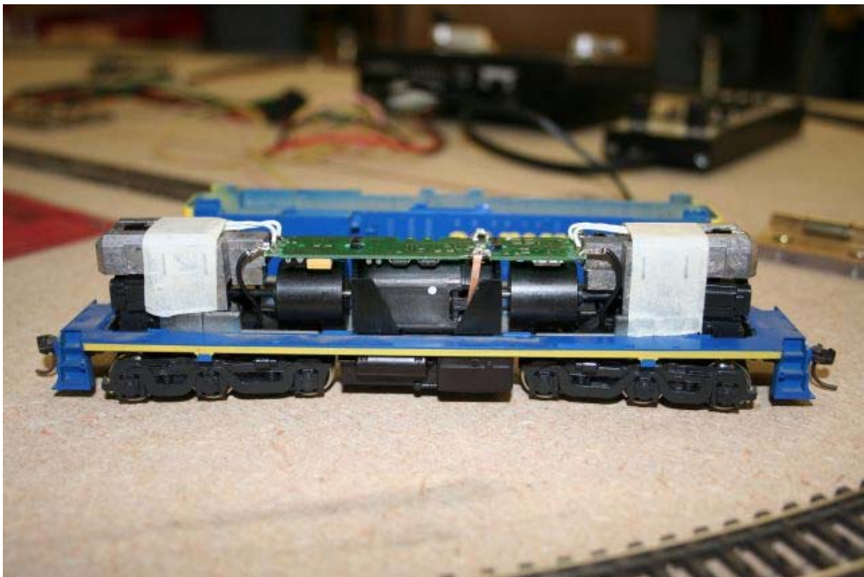
Atlas (Kato) RS1 fitted with Digitrax PnP DH150 decoder during the presentation
